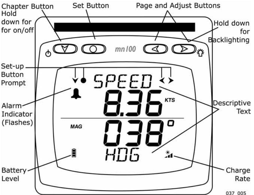
If there is no boat speed or change in heading registered on the system for a period of 12 hours your Micronet instrument will switch off to conserve power. A "POWER SAVE" alarm will sound before the instrument system is switched off. Pressing any button within 10 seconds of the alarm sounding will allow the system to remain switched on.
