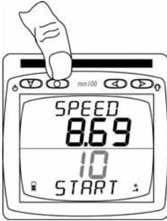
*Press and hold for 1 second to enter the timer setup*
